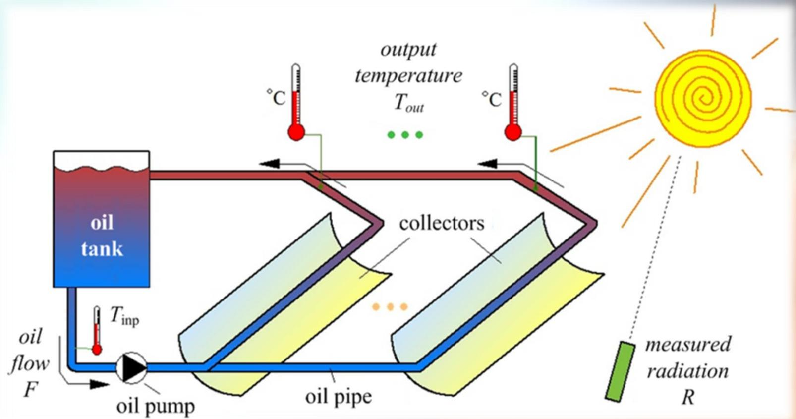
The action on the **pump's flow** changes the residence time of the oil inside the active part of the field, changing the **output temperature**.
